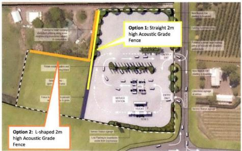
Figure 4: Recommended location of acoustic timber fence options. Not to Scale. Reference: Development Nous.
