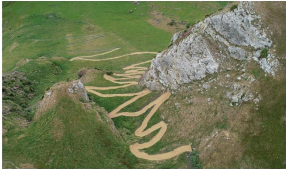
Figure 5: Drone Photograph of coconut (BioCair) matting covered emergency works from above 9/11/2018
