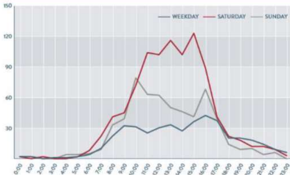
Figure 2-7: Traffic Flow Profile on Te Mata Peak Road (Lower) (June 2018)
