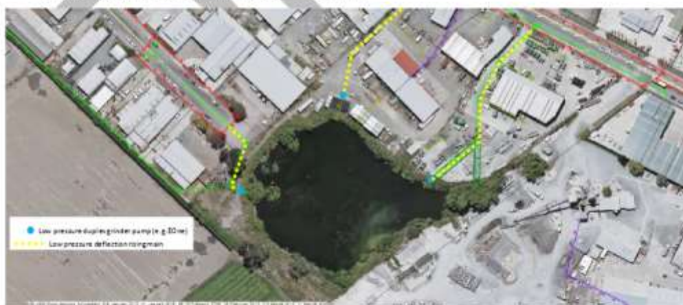
Figure 6.8: General layout of first flush deflection pump back system
