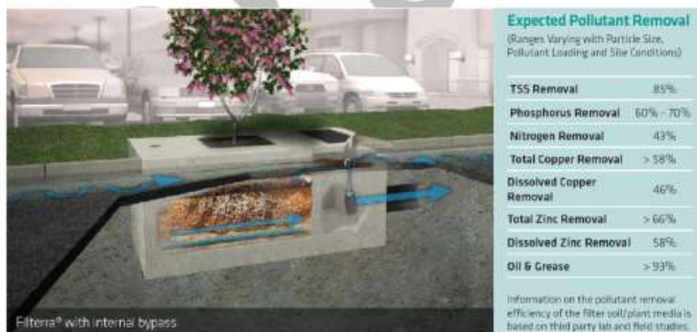
Figure 6.2: Concept layout and treatment efficiency for Stormwater 360 Filterra roadway treatment systems
