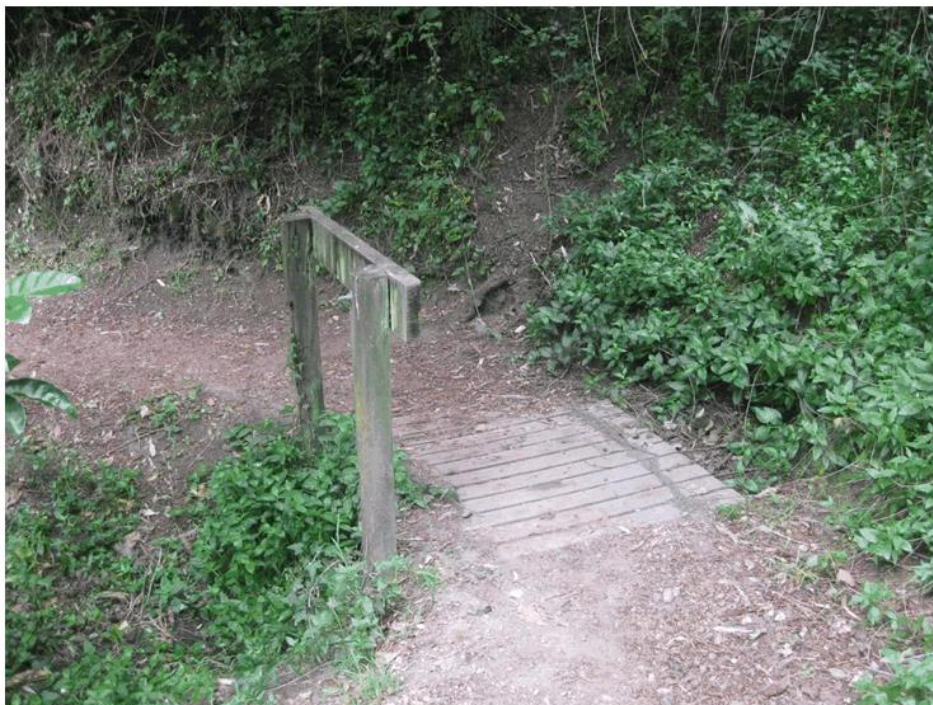
Un-necessary structures should be avoided. A culvert would suffice here.
