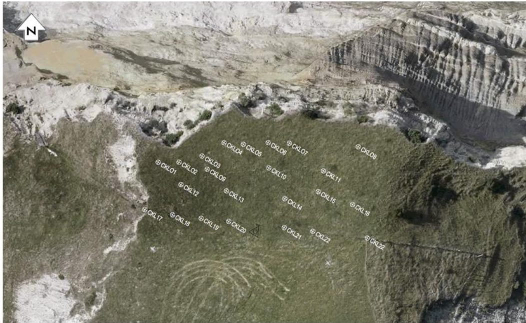
Figure 5-1: Locations of the survey monitoring points located at the cliff top, above the CKL location (5 February 2019)
