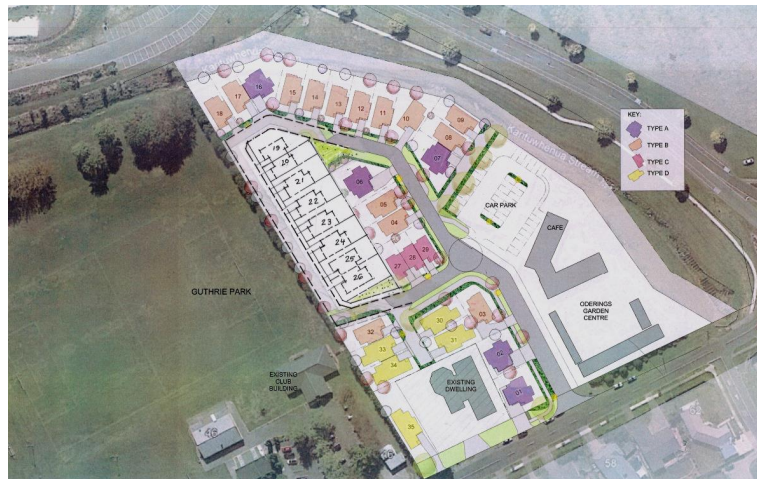
Fig 2: Roading layout with an 'edge lane' along the park frontage / indicative sketch diagram
