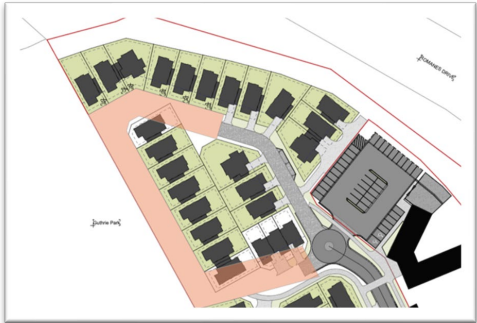
CAD detail showing the impacts of an edge-lane resulting in the loss of two dwellings and compromising (potential loss) of the terraced dwellings.
