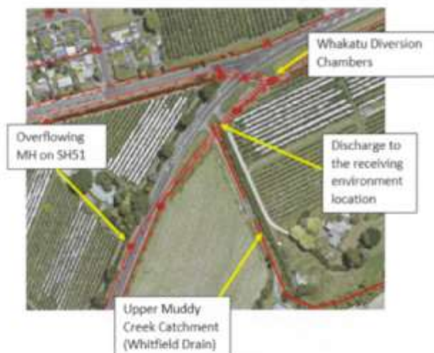
Figure 4: Whakatu wastewater overflow site & discharge to environment site
