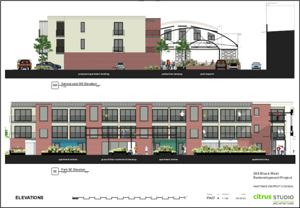
Figure 10: Service Yard South-West Elevation and Park South-East Elevation
