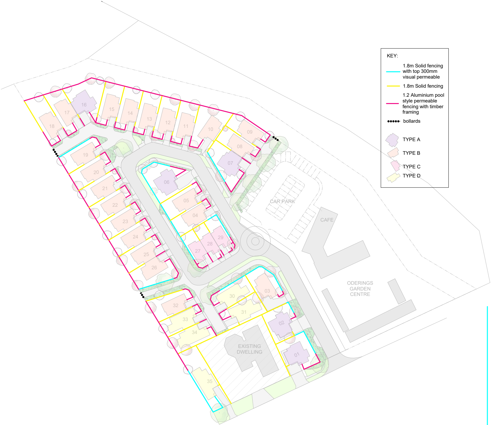
Boundary fencing 1.8m high top 300mm visually permeable- with butted board or hit and miss closed fencing to create privacy between properties and main public spaces with cap and posts exposed on both sides, kickboards optional but match close boundary fencing. Permeable section with every second board missing or chunky horizontal rungs if main boundary fencing has kick and top board. Gates to match
