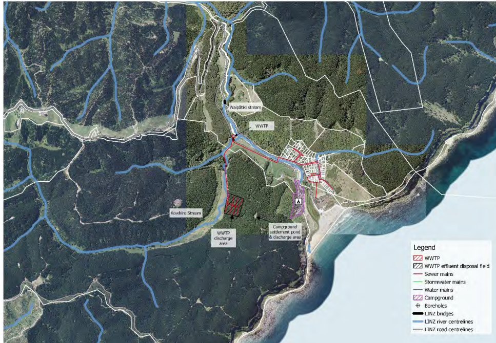
Figure 2: Site plan showing property boundaries (white lines) and three waters infrastructure for campground and community WWTP
