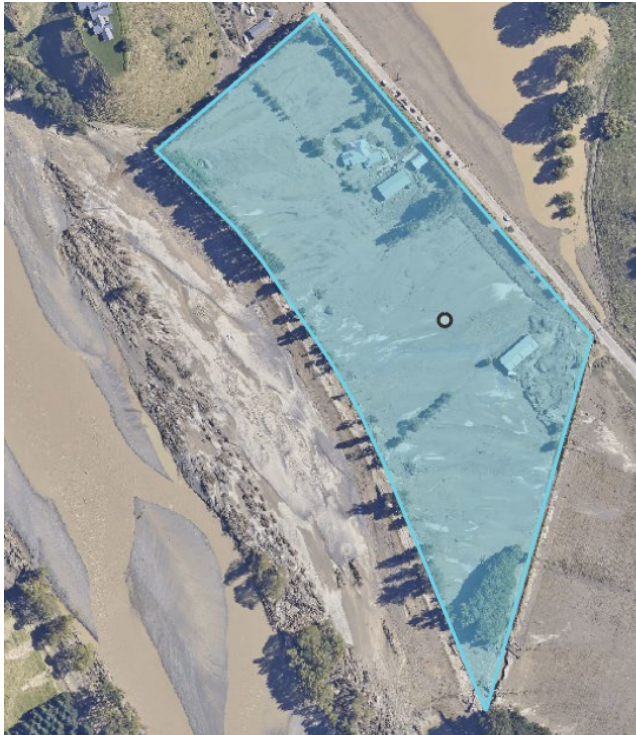
FIGURE 4: IMAGE OF 613 PUKETAPU ROAD DAYS AFTER CYCLONE GABRIELLE SHOWING COMPLETE SILT INUNDATION.
