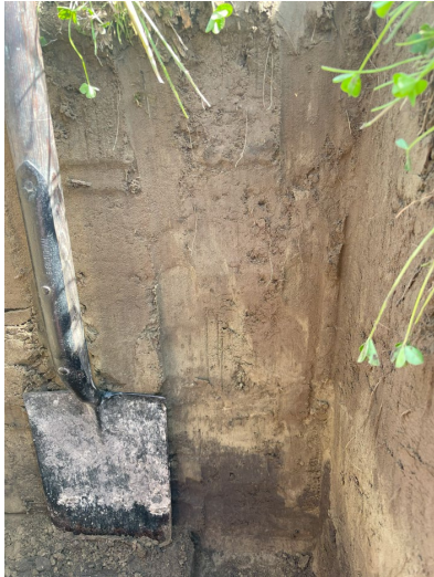
FIGURE 10: SOIL PIT DUG AT NORTHERN END OF SITE. DEPOSITED FINE SAND SITS ON TOP OF BURIED SOIL PROFILE AT BOTTOM OF PIT. APPARENT CHANGE IN COLOUR DOWN THE PROFILE IS A WETTED FRONT FOLLOWING RECENT RAINFALL AFTER A VERY DRY SPRING. WHEN DRY THIS SOIL IS THE SAME PALE COLOUR AS EVIDENT ABOVE THE BURIED TOPSOIL.
