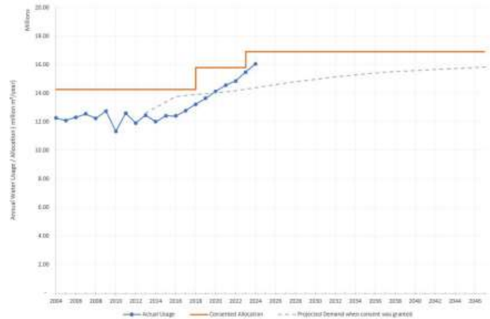
FIGURE 44: HASTINGS URBAN WATER SUPPLY – CONSENT ALLOCATION VS ACTUAL USAGE
